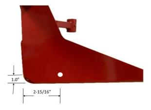
3. Measurements for the holes in the sides of the pan:
